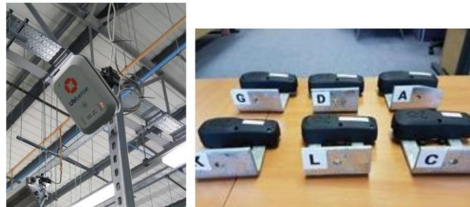
Current Converter and Toroidal Hardware Implemented to Capture Welding Current
